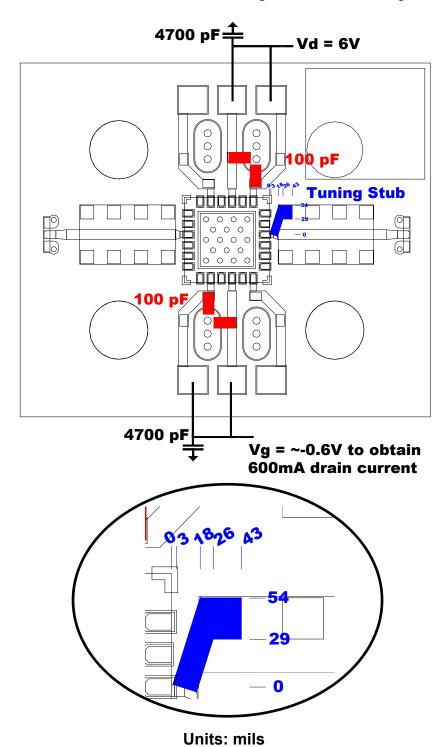
\* This layout shows the tuning configuration used to obtain the measured data. The layout configuration may vary depending on the specific application.
